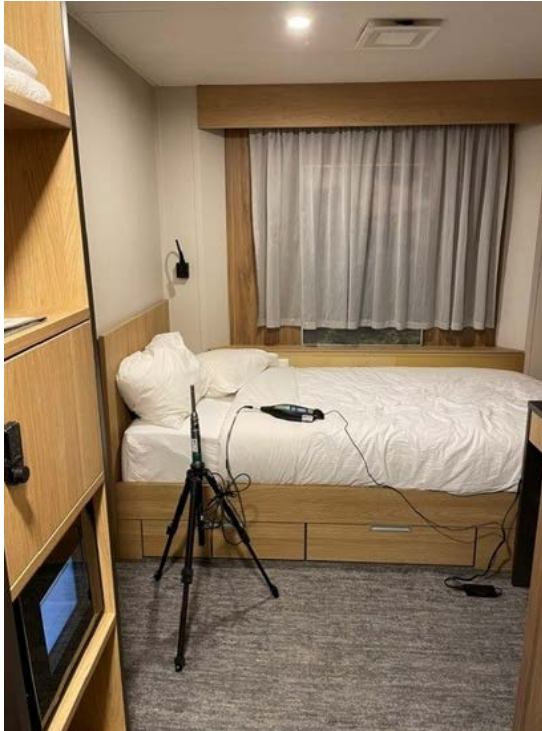
Figure 7 Sound Level Meter Setup at Cabin 5645 – Floatel #1
