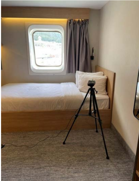
Figure 10 Sound Level Meter Setup at Cabin 9215 – Floatel #1
