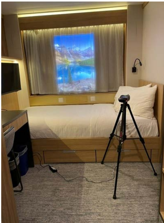
Figure 8 Sound Level Meter Setup at Cabin 6637 – Floatel #1
