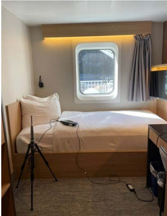
Figure 11 Sound Level Meter Setup at Cabin 0108 – Floatel #1
