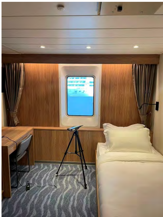
Figure 14 Sound Level Meter Setup at Cabin 064 – Floatel #2
