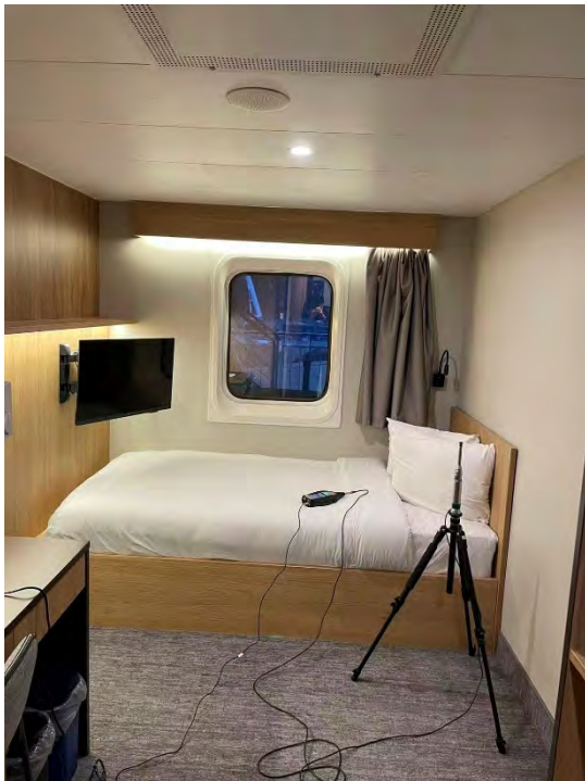
Figure 10 Sound Level Meter Setup at Cabin 9400 – Floatel #1
