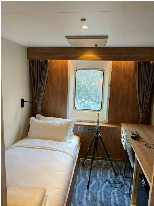
Figure 12 Sound Level Meter Setup at Cabin 4482 – Floatel #2
