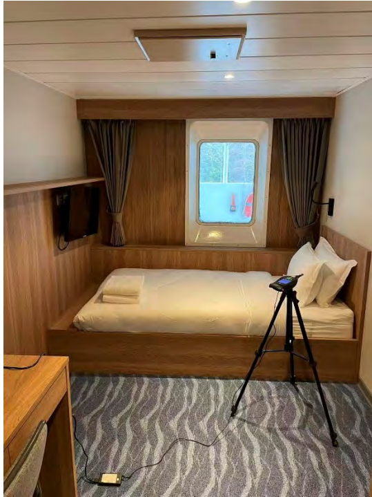
Figure 13 Sound Level Meter Setup at Cabin 508 – Floatel #2
