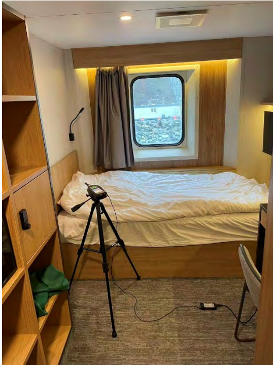
Figure 7 Sound Level Meter Setup at Cabin 5628 – Floatel #1
