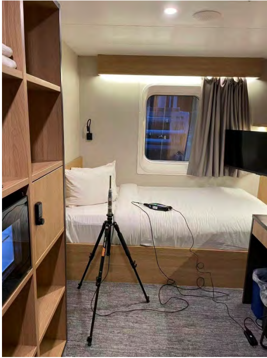
Figure 11 Sound Level Meter Setup at Cabin 0102 – Floatel #1
