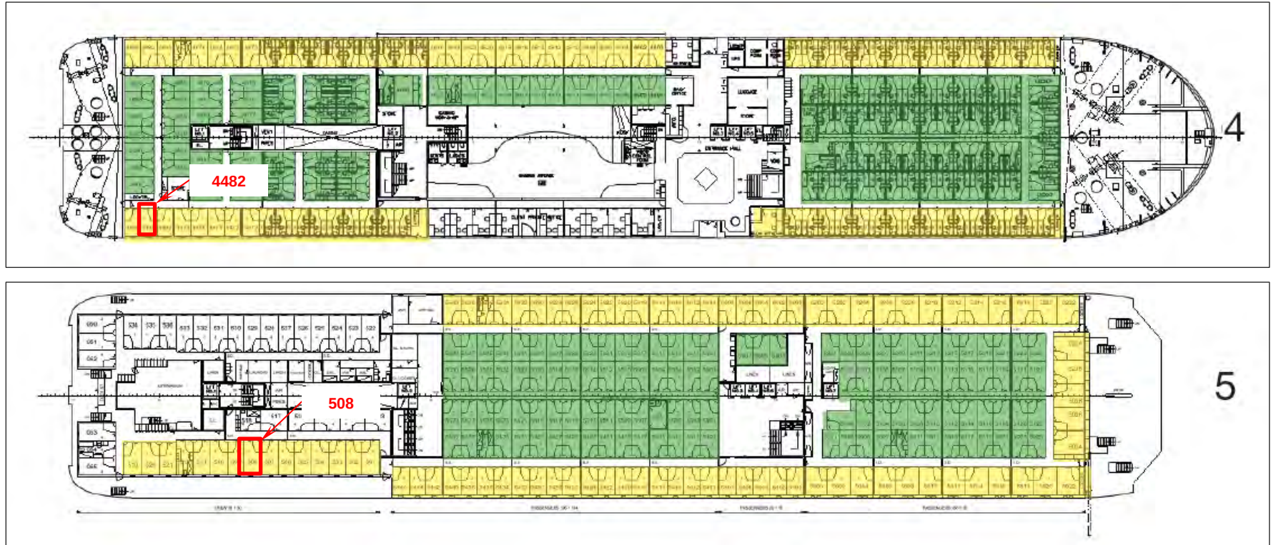
Figure 5 Measurement Location at Cabin 4482 and Cabin 508 (Deck 4 and Deck 5) – Floatel #2
