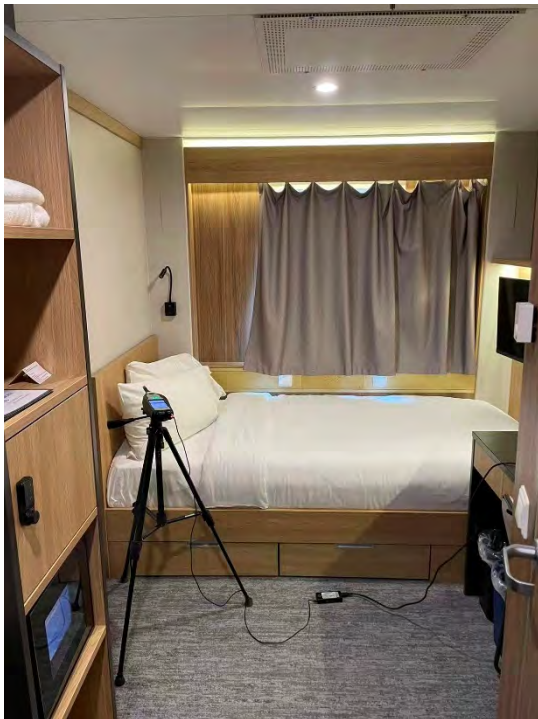
Figure 8 Sound Level Meter Setup at Cabin 6622 – Floatel #1
