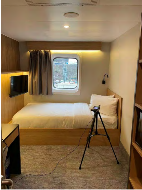
Figure 9 Sound Level Meter Setup at Cabin 7004 – Floatel #1
