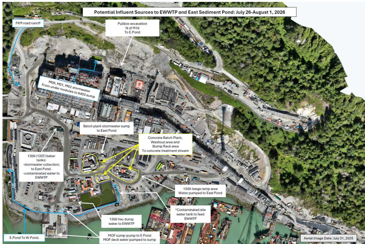
Figure 2: East Catchment contact water management facilities (July 26 – August 1).
