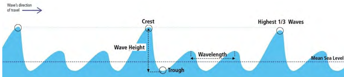
Figure 3 Graphical wave height definition
