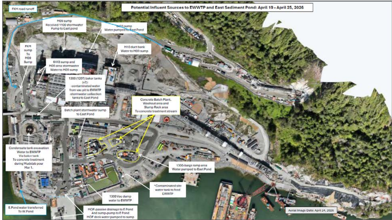
Figure 2: East Catchment contact water management facilities (April 19 – 25).
