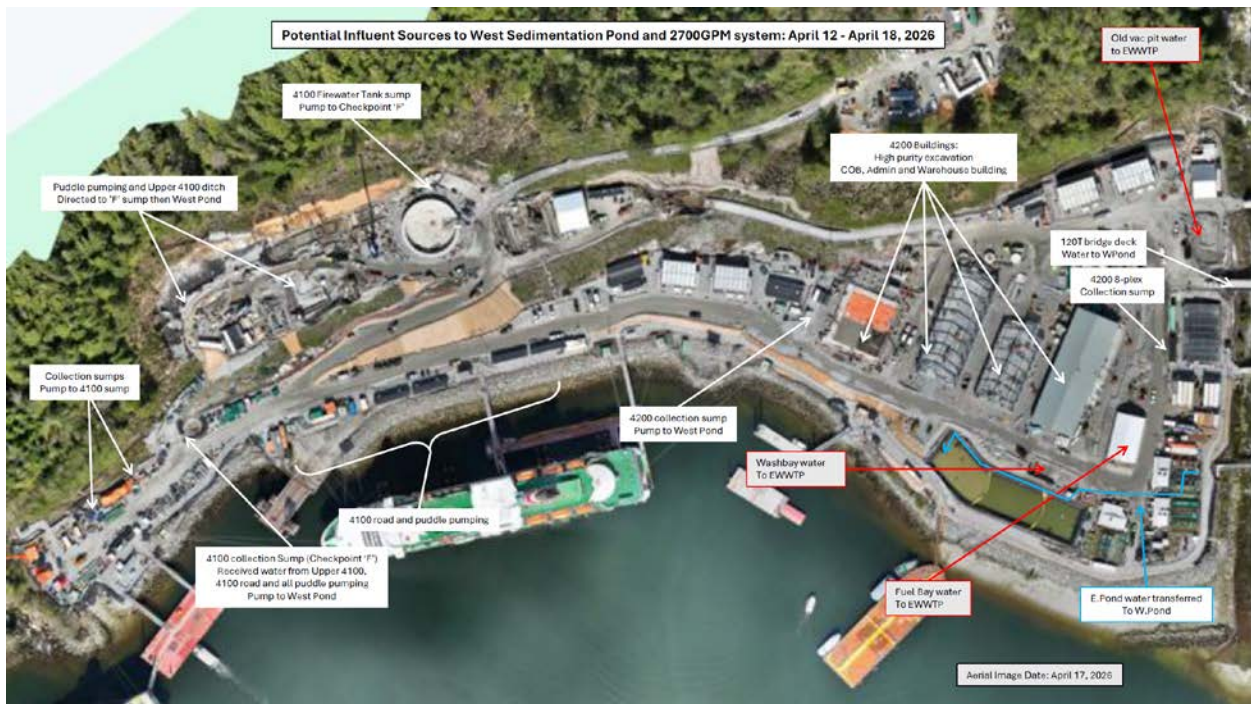
Figure 3: West Catchment contact water management facilities (April 12 – 18).
