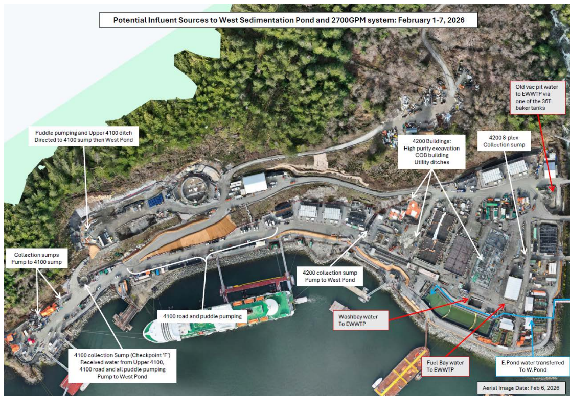
Figure 3: West Catchment contact water management facilities (February 1 – 7).
