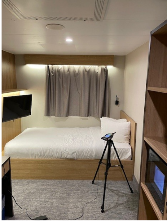
Figure 10 Sound Level Meter Setup at Cabin 0105
