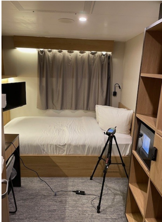
Figure 10 Sound Level Meter Setup at Cabin 0105
