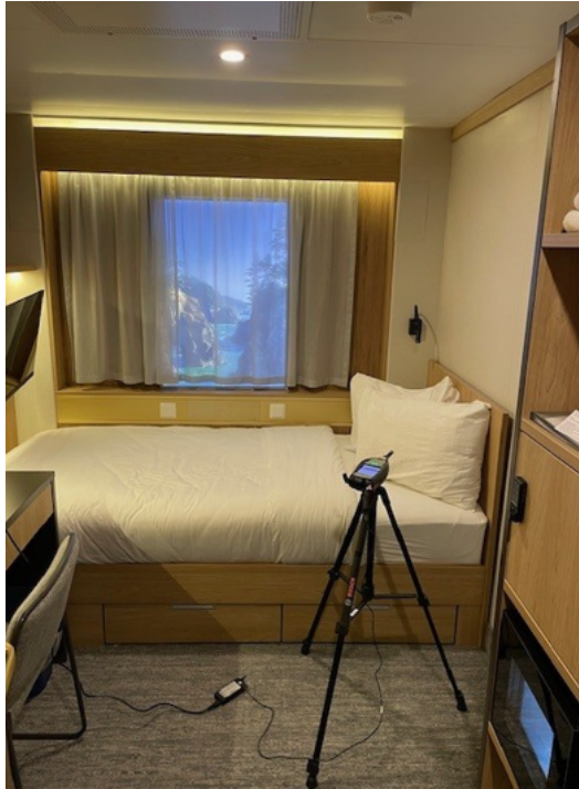
Figure 6 Sound Level Meter Setup at Cabin 5634
