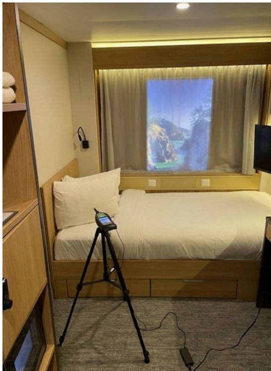
Figure 8 Sound Level Meter Setup at Cabin 7716
