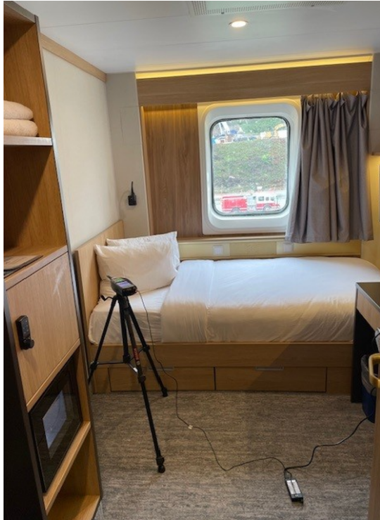
Figure 8 Sound Level Meter Setup at Cabin 7716
