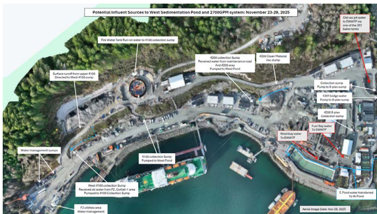
Figure 3: West Catchment contact water management facilities (November 23 - 29).
