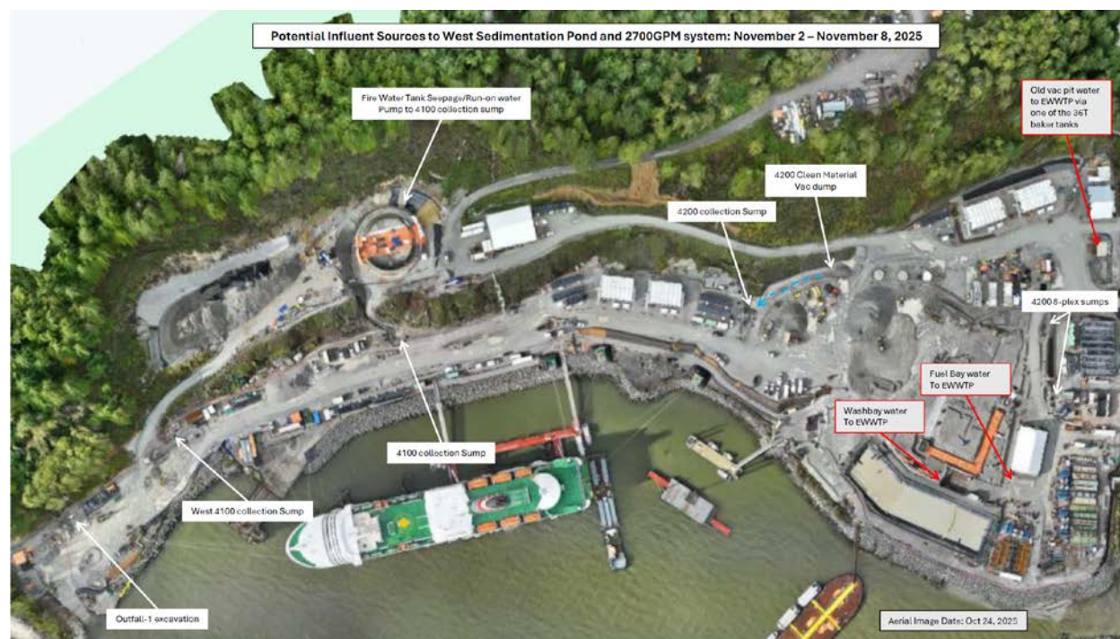
Figure 3: West Catchment contact water management facilities (November 2 - 8).
