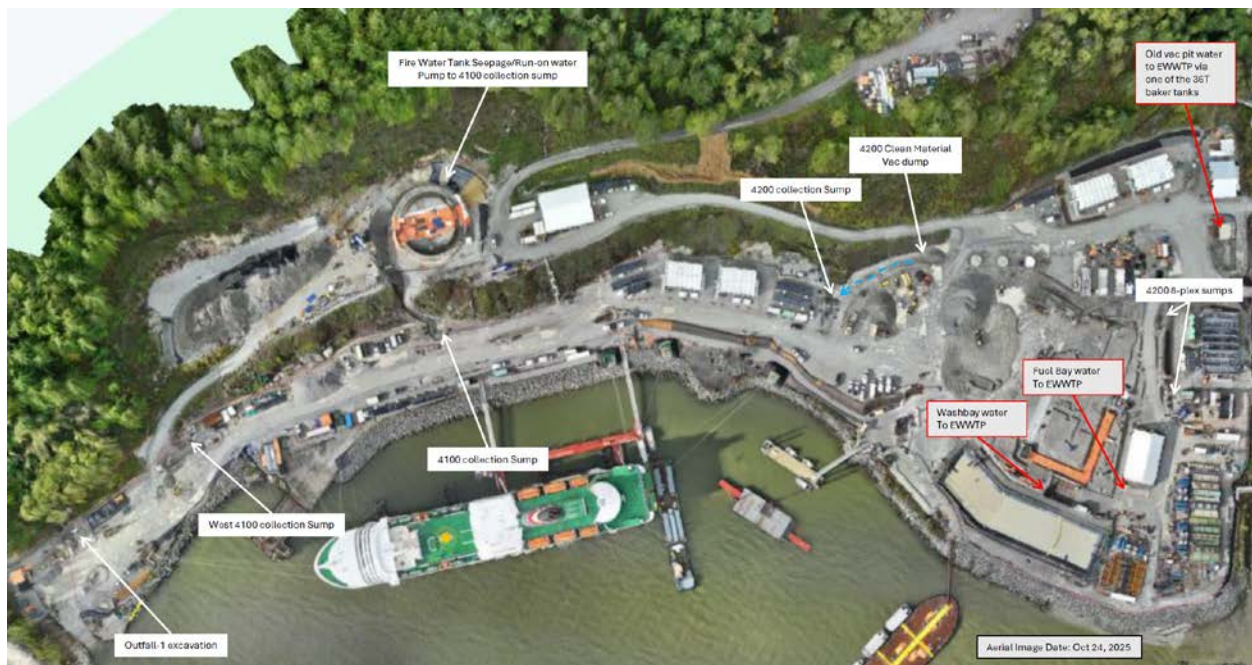
Figure 3: West Catchment contact water management facilities (October 26 – November 1).
