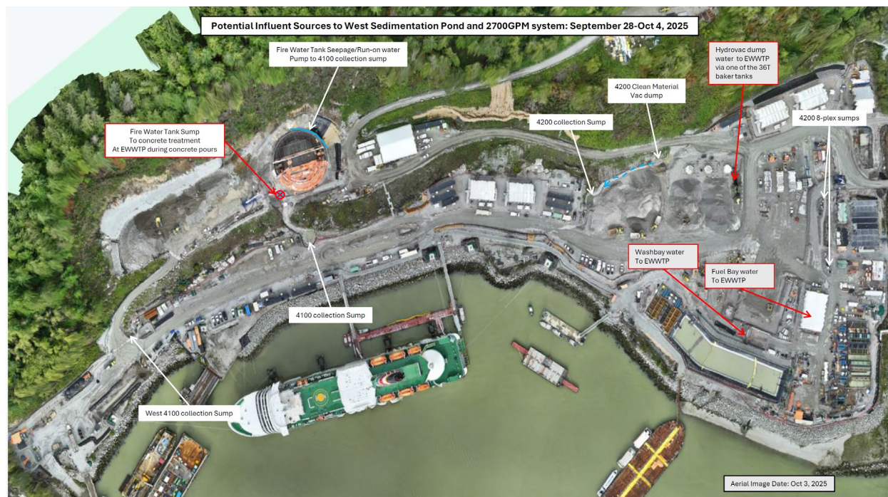
Figure 3: West Catchment contact water management facilities (September 28 – October 4).
