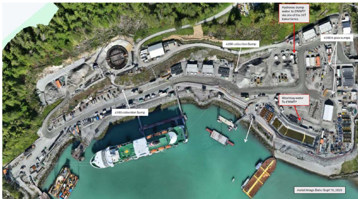
Figure 3: West Catchment contact water management facilities (September 21 – 27).
