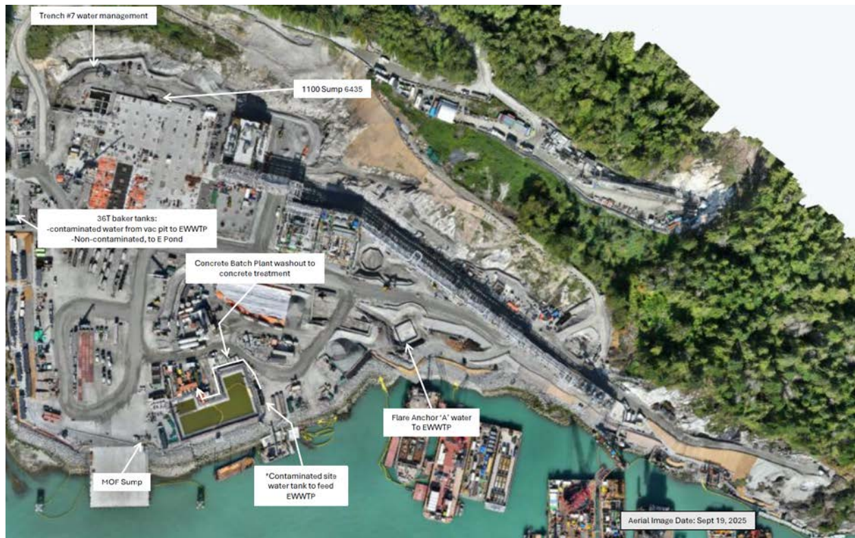
Figure 2: East Catchment contact water management facilities (September 21 – 27).
