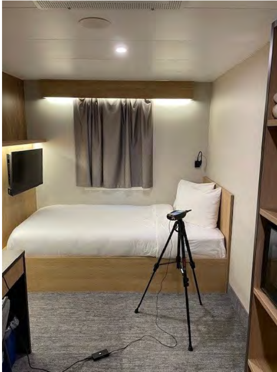
Figure 10 Sound Level Meter Setup at Cabin 0108
