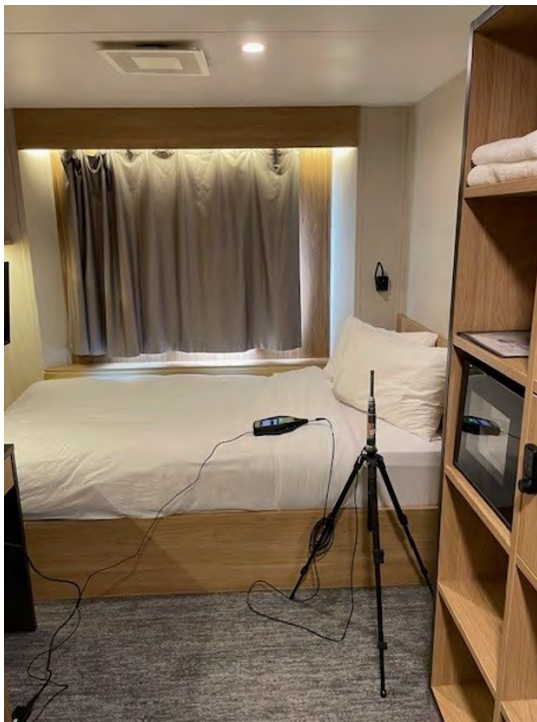
Figure 6 Sound Level Meter Setup at Cabin 5616
