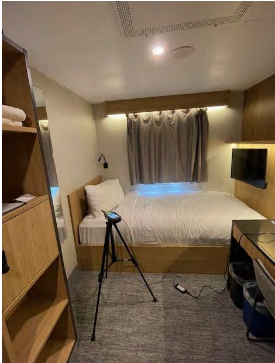
Figure 10 Sound Level Meter Setup at Cabin 0108
