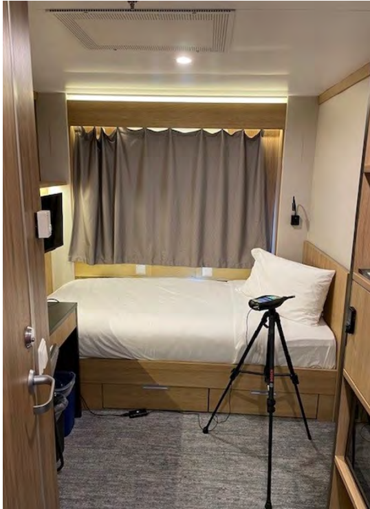
Figure 8 Sound Level Meter Setup at Cabin 7028
