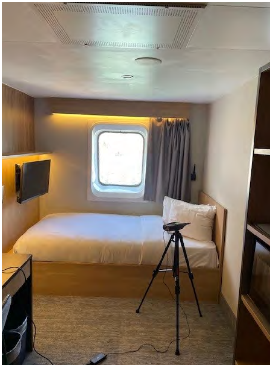
Figure 8 Sound Level Meter Setup at Cabin 7028
