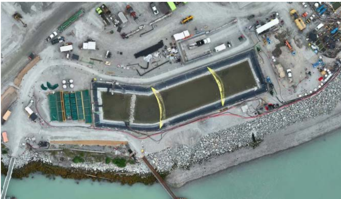
Figure 5: Aerial view of the West Sedimentation Pond (July 18, 2025). The 2700GPM TSS settling system is located to the left of the pond. Algal mats are visible in the centre and final cells of the pond.
