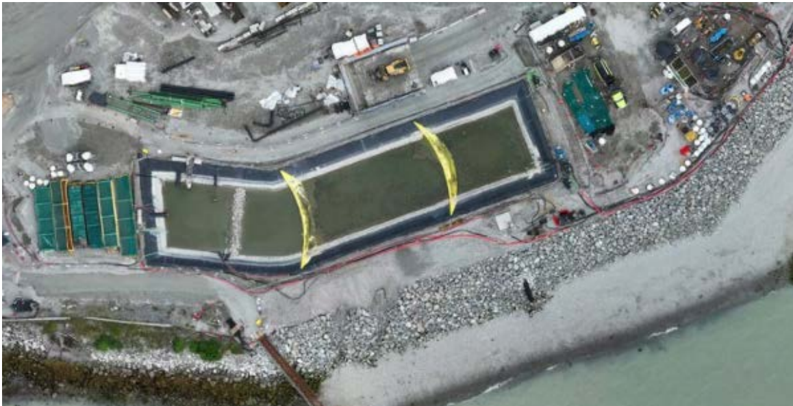
Figure 5: Aerial view of the West Sedimentation Pond (July 10, 2025). The 2700GPM TSS settling system is located to the left of the pond. Algal mats are visible in the centre and final cells of the pond.
