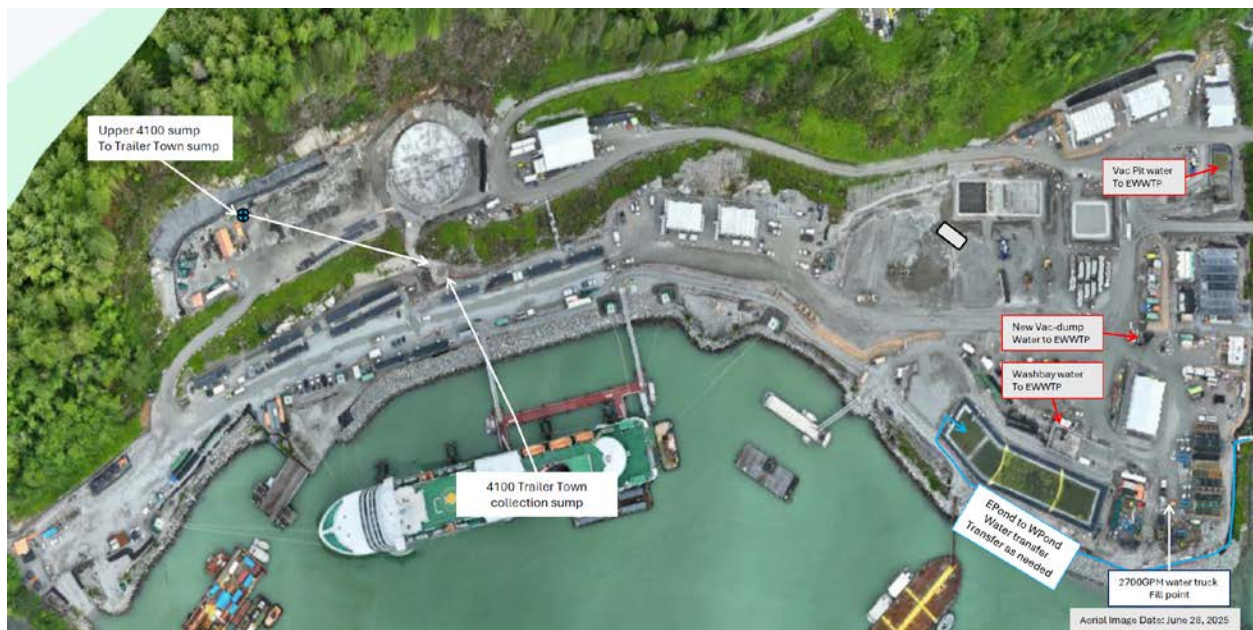
Figure 3: West Catchment contact water management facilities (June 29 – July 5).
