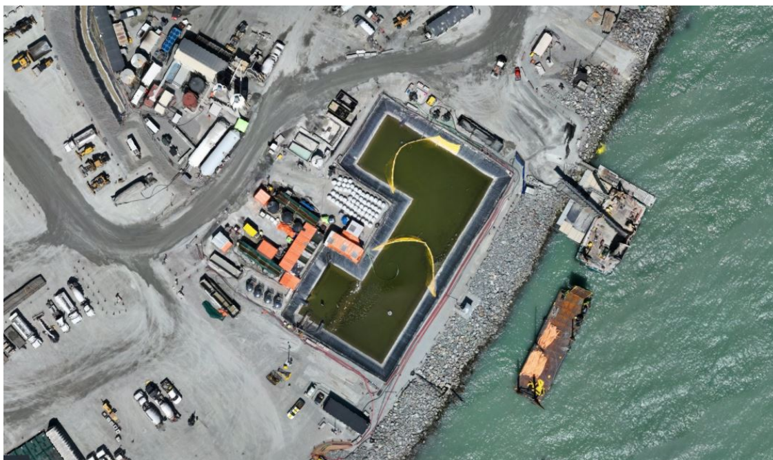
Figure 4: Aerial view of the East Sedimentation Pond (July 4, 2025). The East WWTP is located on the left side and the E500GPM TSS settling system is situated along the bottom edge of the pond. Algal mats are visible in the central cell of the pond.
