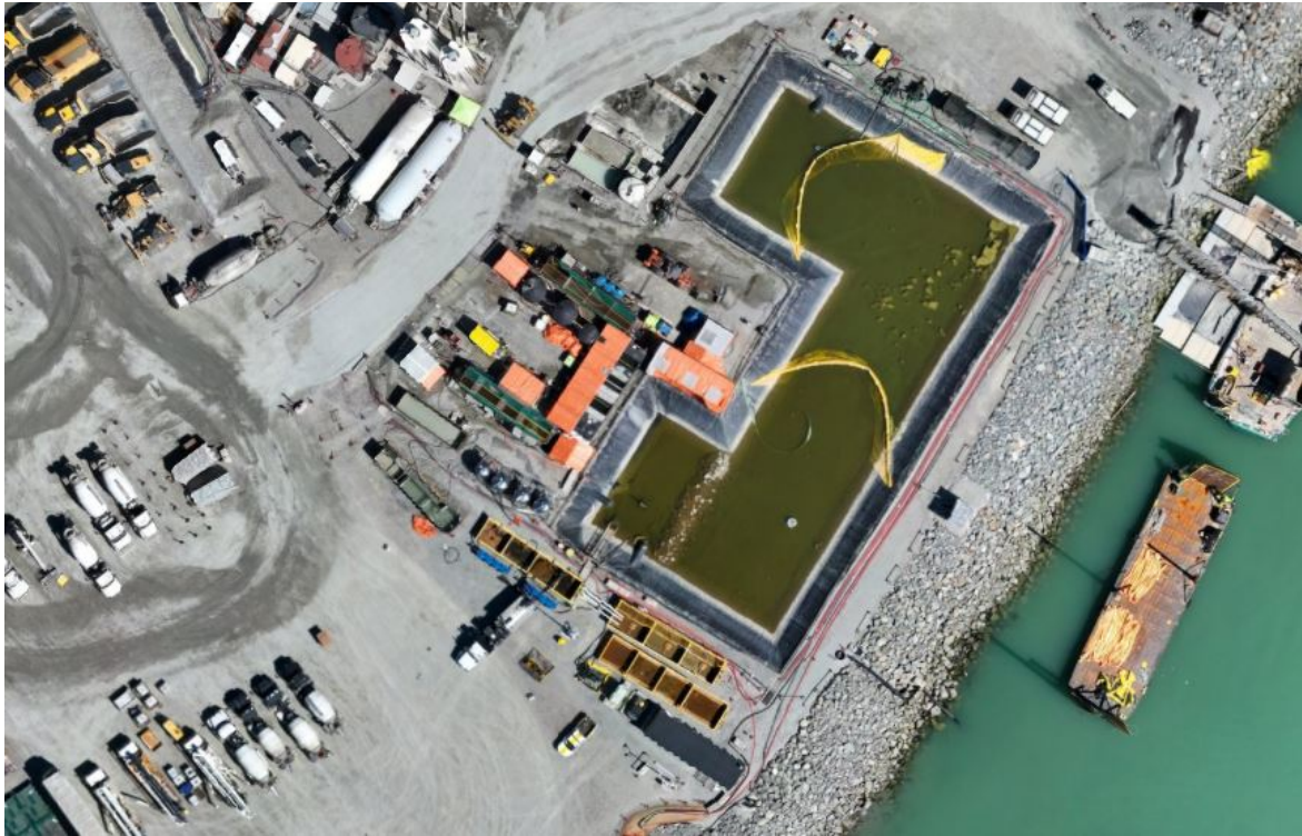
Figure 4: Aerial view of the East Sedimentation Pond (June 28, 2025). The East WWTP is located on the left side and the E500GPM TSS settling system is situated along the bottom edge of the pond. Algal mats are visible in the central cell of the pond.
