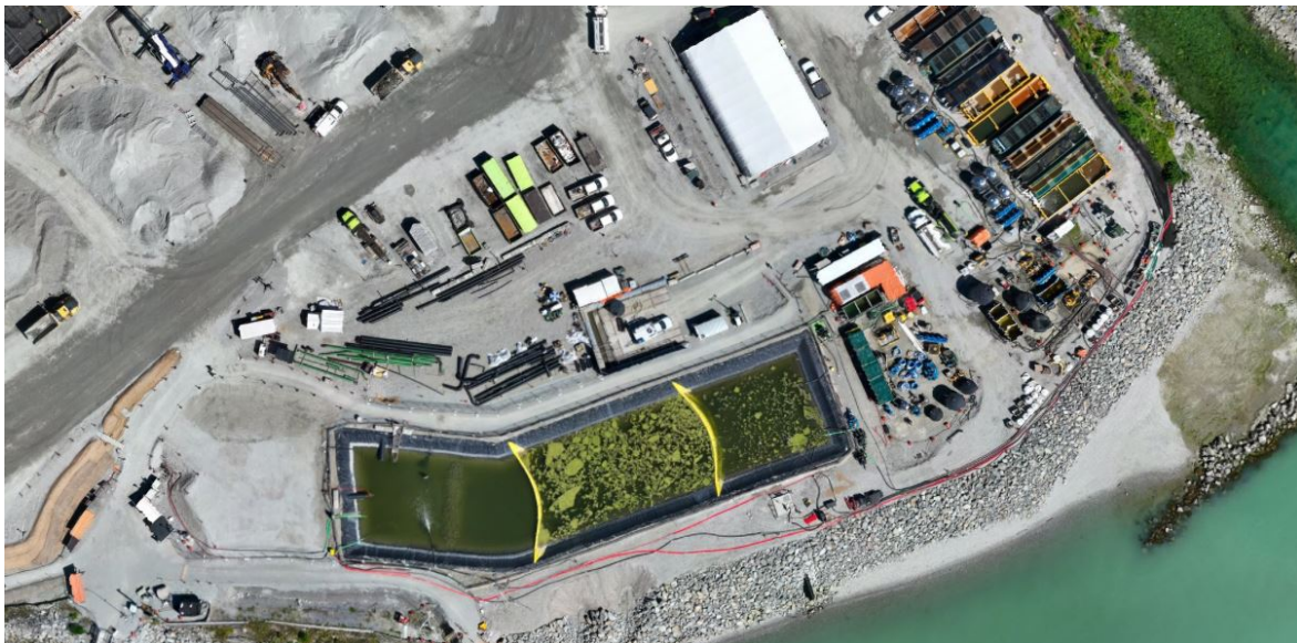
Figure 5: Aerial view of the West Sedimentation Pond (June 28, 2025). The TSS settling systems are located to the left (W500GPM) and right (ESC) of the pond. Algal mats are visible in the centre and final cells of the pond.
