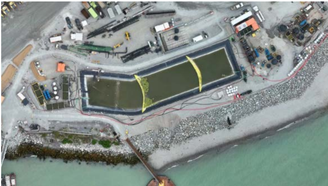
Figure 5: Aerial view of the West Sedimentation Pond (June 13, 2025). The TSS settling systems are located to the left (W500GPM) and right (ESC) of the pond.
