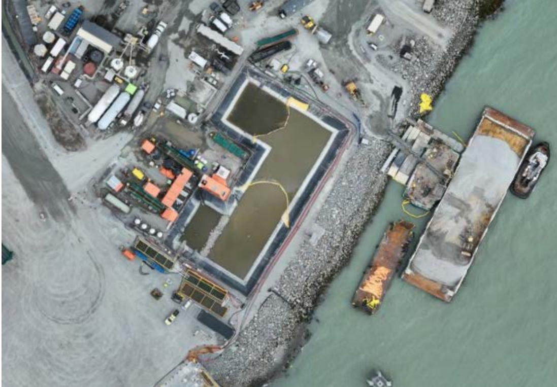
Figure 4: Aerial view of the East Sedimentation Pond (June 13, 2025). The East WWTTP is located on the left side and the E500GPM TSS settling system is situated along the bottom edge of the pond.
