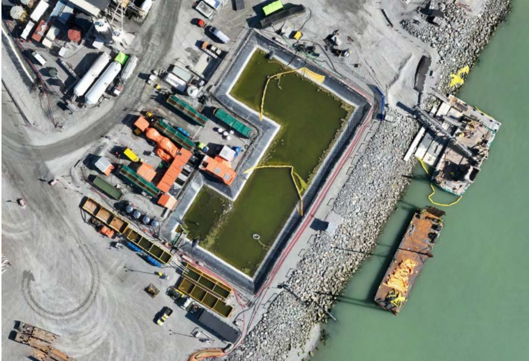
Figure 4: Aerial view of the East Sedimentation Pond (June 6, 2025). The East WWT is located on the left side and the E500GPM TSS settling system is situated along the bottom edge of the pond.
