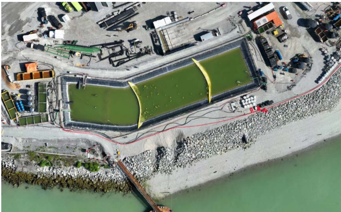
Figure 5: Aerial view of the West Sedimentation Pond (June 6, 2025). The TSS settling systems are located to the left (W500GPM) and right (ESC) of the pond.
