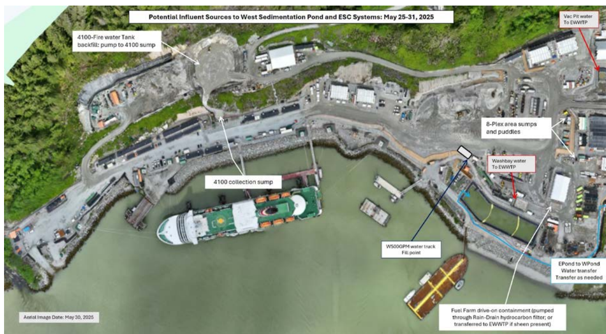
Figure 3: West Catchment contact water management facilities (May 25 - 31).
