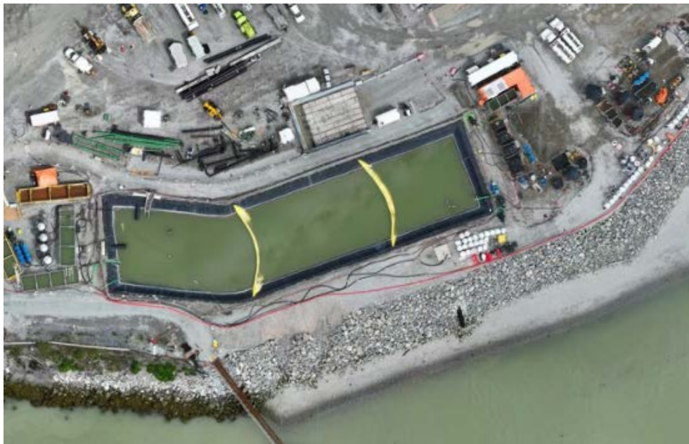
Figure 5: Aerial view of the West Sedimentation Pond (May 30, 2025). The TSS settling systems are located to the left (W500GPM) and right (ESC) of the pond.
