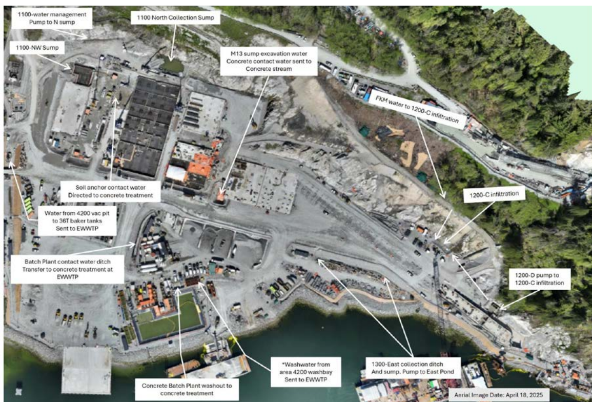
Figure 2: East Catchment contact water management facilities (April 20 – 26).
