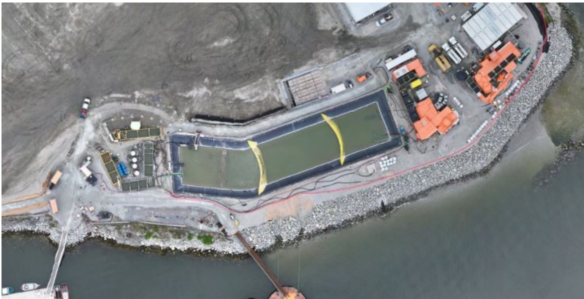
Figure 5: Aerial view of the West Sedimentation Pond (April 25, 2025). The TSS settling systems are located to the left (W500GPM) and right (ESC) of the pond.
