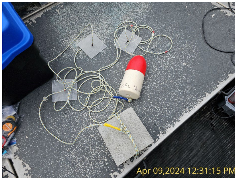
Photograph A22: Aquatic Invasive Species Collector Plate Array Deployed at the North Reference Site. Each collector plate included a marker buoy attached to lead-core sinking rope line. Sanded PVC plates were threaded on the rope line and secured at desired depths with zip ties. Each array was weighted at the bottom with a concrete cinder block.
