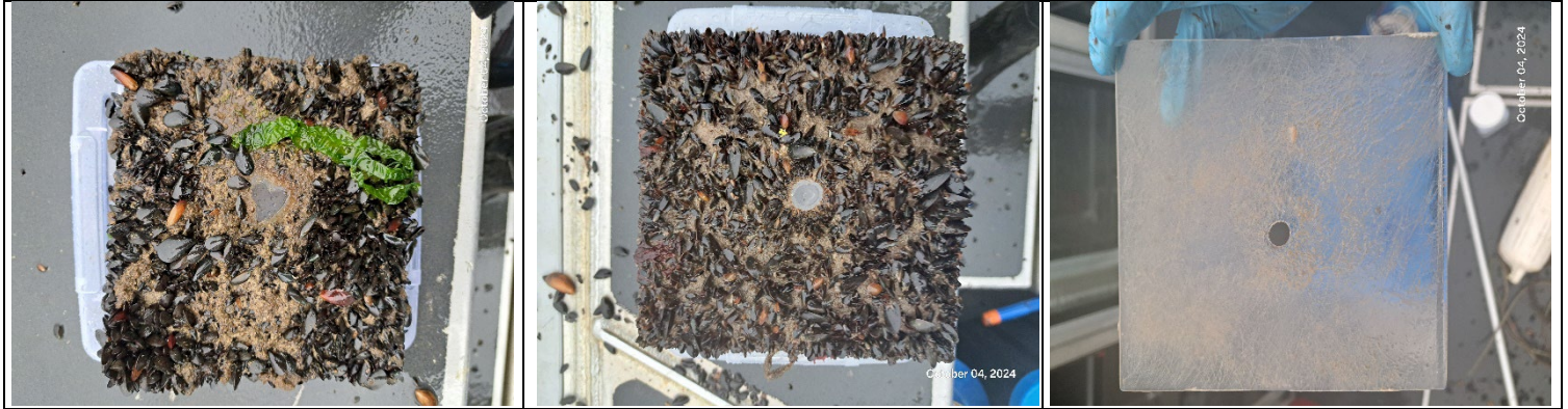
Photograph A23: Aquatic Invasive Species Collector Plates deployed April 9, 2024, and collected October 4, 2024, at AIS-1 (in proximity to Woodfibre Creek and Ro-Ro). The top plate (left) was deployed 1 m below the water surface, the middle plate (middle) was deployed 5 m below the water surface, and the bottom plate (right) was deployed 6 m below the water surface.
