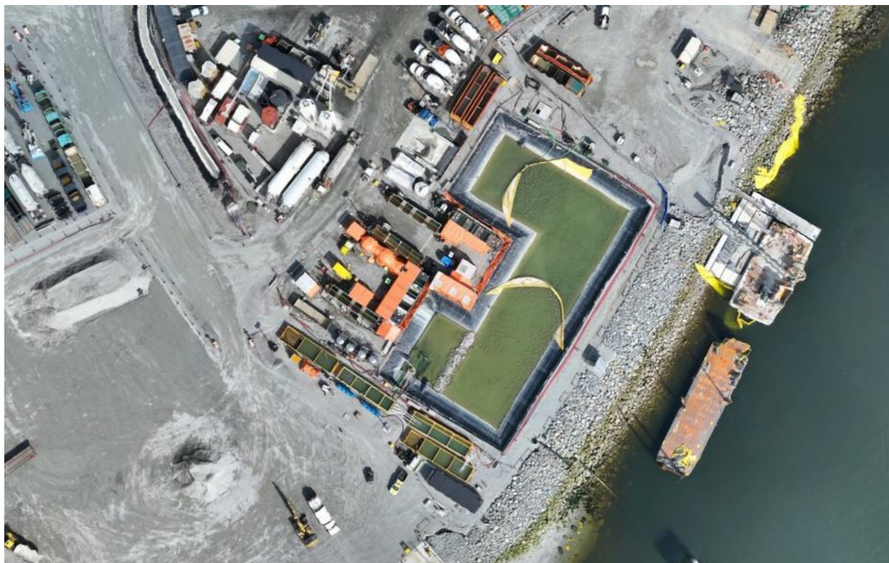
Figure 4: Aerial view of the East Sedimentation Pond (April 9, 2025). The East WWTP is located on the left side and the E500GPM TSS settling system is situated along the bottom edge of the pond.
