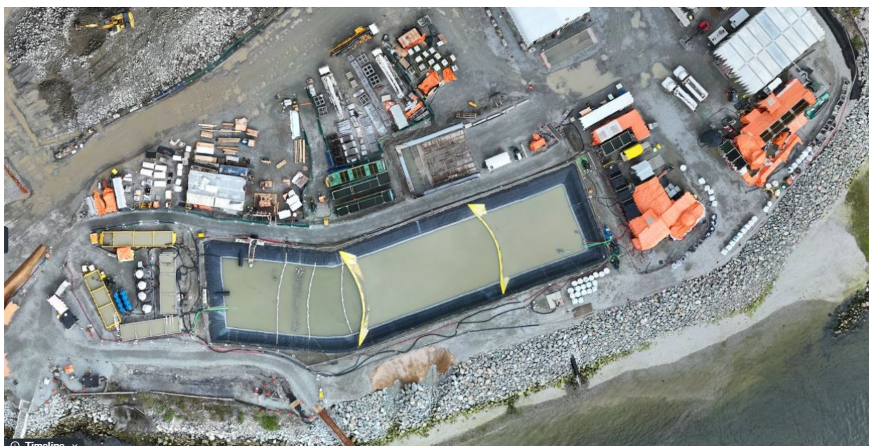
Figure 5: Aerial view of the West Sedimentation Pond (April 9, 2025). The TSS settling systems are located to the left (W500GPM) and right (ESC) of the pond.
