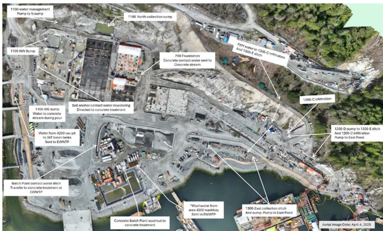
Figure 2: East Catchment contact water management facilities (April 6 – 12).
