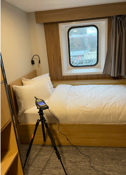
Figure 6 Sound Level Meter Setup at Cabin 5632
