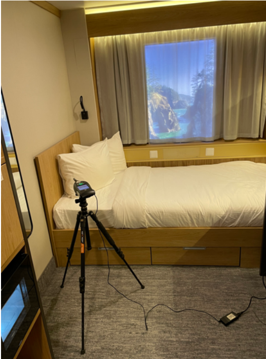
Figure 6 Sound Level Meter Setup at Cabin 5632
