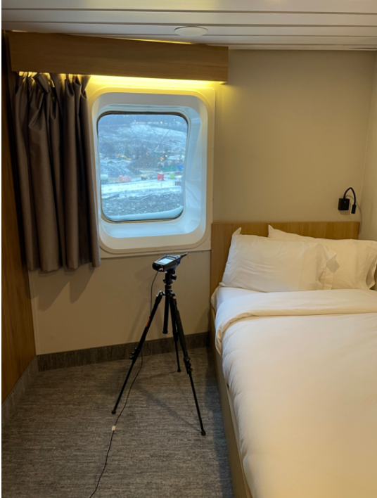
Figure 8 Sound Level Meter Setup at Cabin 7024
