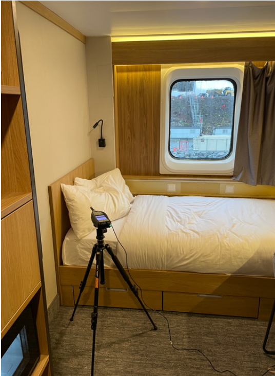
Figure 8 Sound Level Meter Setup at Cabin 7024
