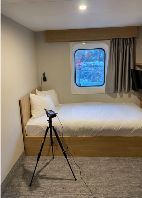
Figure 10 Sound Level Meter Setup at Cabin 0103
