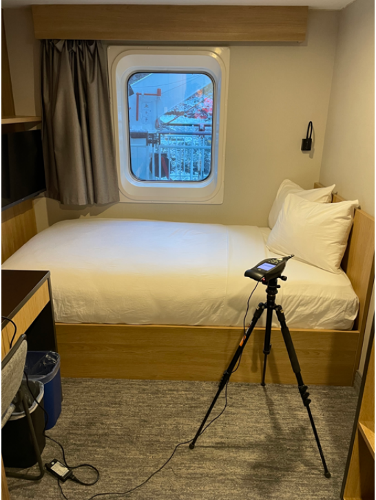
Figure 10 Sound Level Meter Setup at Cabin 0103
