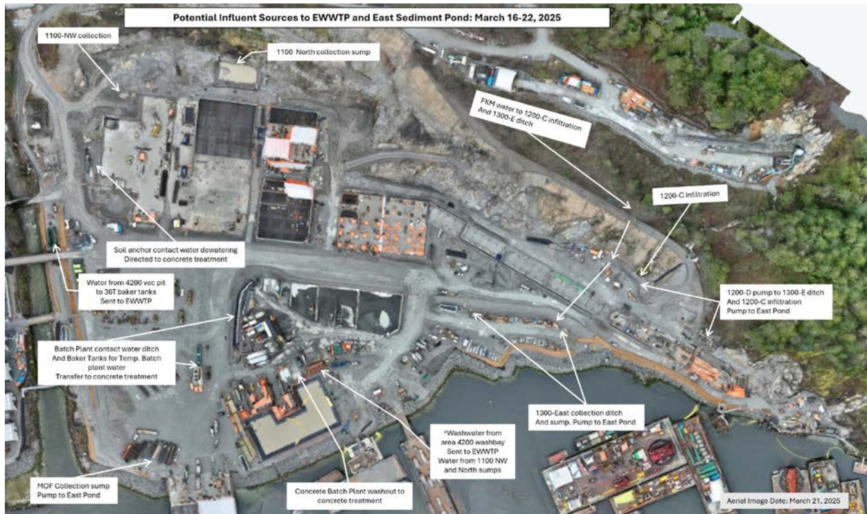
Figure 2: East Catchment contact water management facilities (March 16 – March 22).
