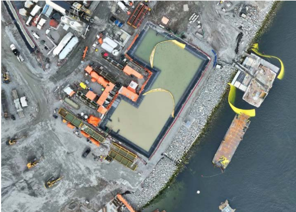
Figure 4: Aerial view of the East Sedimentation Pond (March 13, 2025). The East WWTP is located on the left side and the E500GPM TSS settling system is situated along the bottom edge of the pond.
