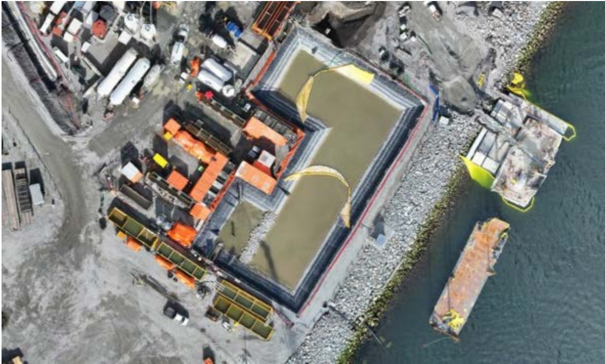
Figure 4: Aerial view of the East Sedimentation Pond (February 28, 2025). The East WWTP is located on the left side and the E500GPM TSS settling system is situated along the bottom edge of the pond.
