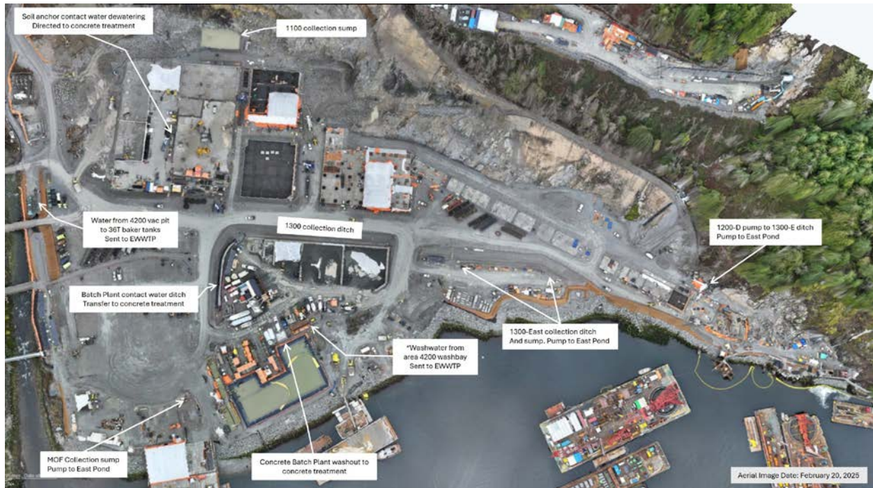
Figure 2: East Catchment contact water management facilities (February 16 – February 22).
