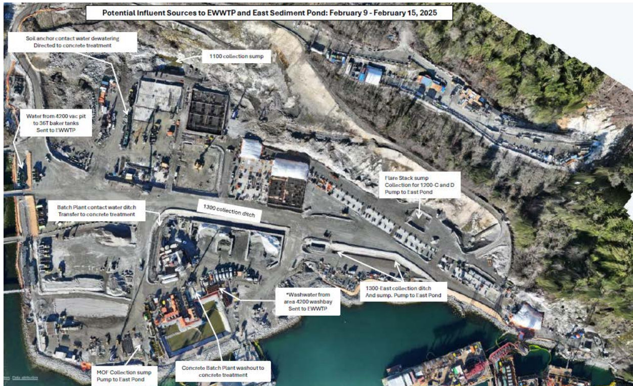
Figure 2: East Catchment contact water management facilities (February 9 – February 15).
