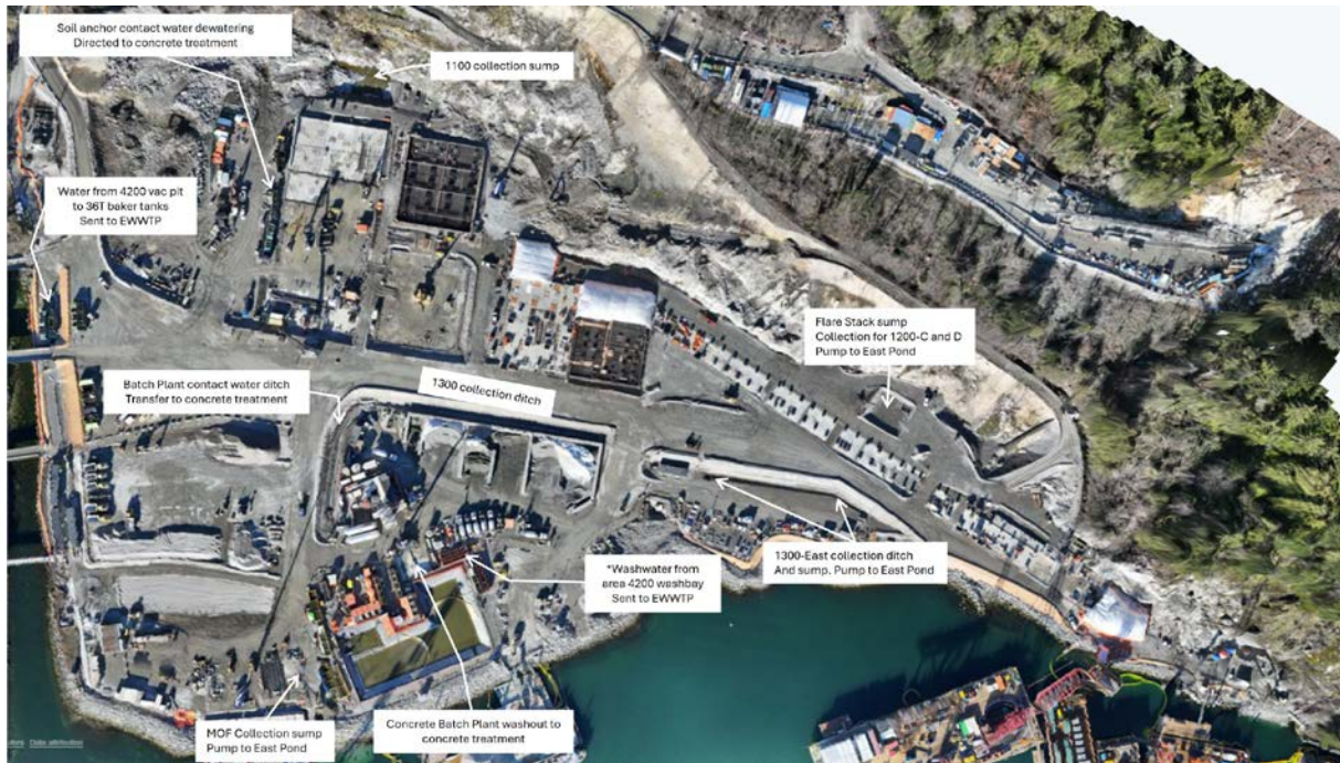
Figure 2: East Catchment contact water management facilities (January 26 – February 1).
