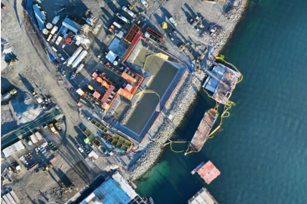
Figure 4: Aerial view of the East Sedimentation Pond (January 17, 2024). The East WWTP is located on the left side and the E500GPM TSS settling system is situated along the bottom edge of the pond.
