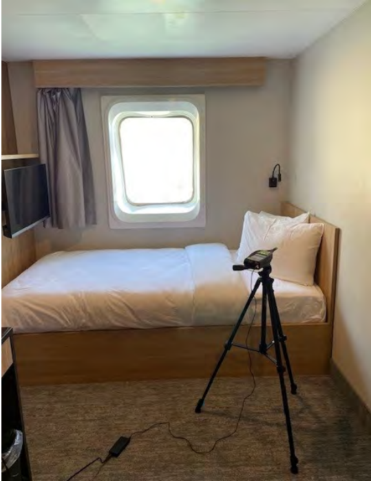
Figure 8 Sound Level Meter Setup at Cabin 7027
