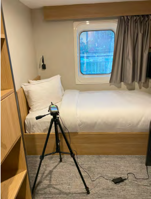
Figure 10 Sound Level Meter Setup at Cabin 0106
