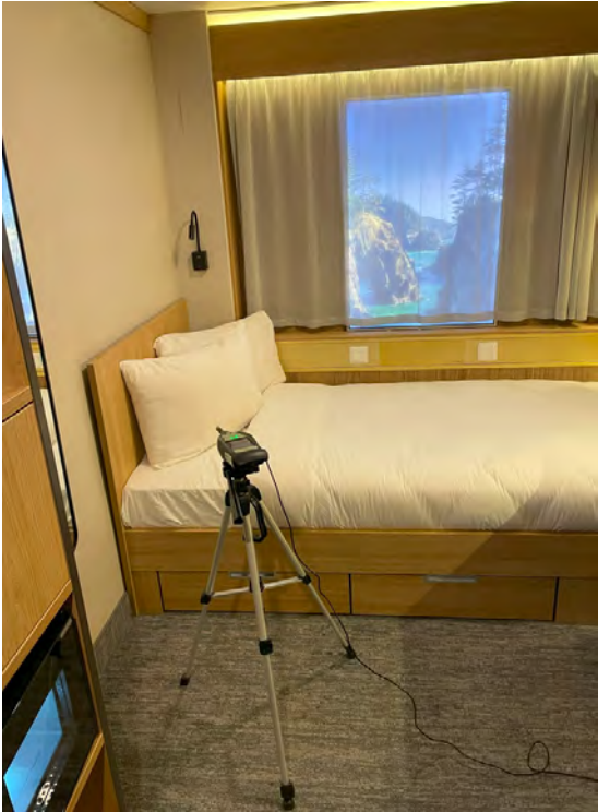
Figure 6 Sound Level Meter Setup at Cabin 5004
