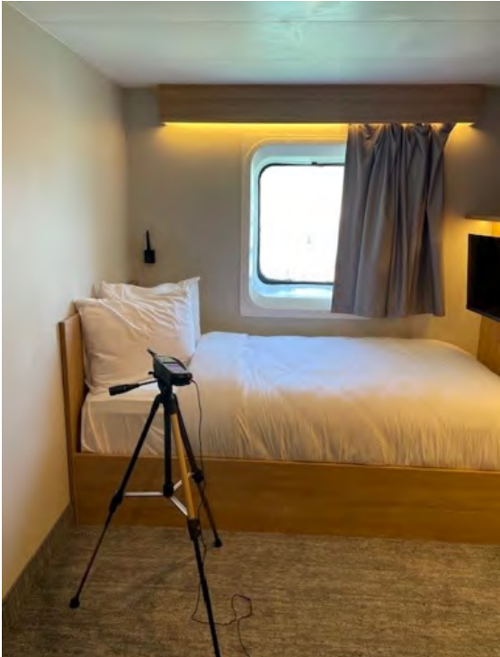
Figure 8 Sound Level Meter Setup at Cabin 9410
