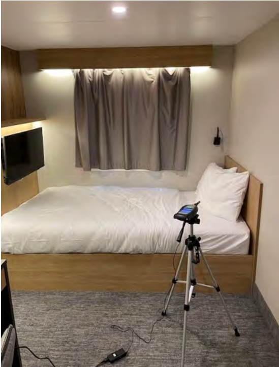
Figure 8 Sound Level Meter Setup at Cabin 9410
