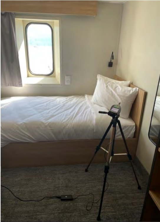
Figure 6 Sound Level Meter Setup at Cabin 6008
