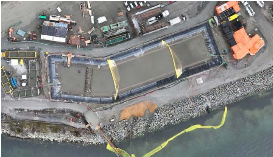
Figure 5: Aerial view of the West Sedimentation Pond (December 6, 2024). The TSS settling systems are located to the left (W500GPM) and right (ESC) of the pond.
