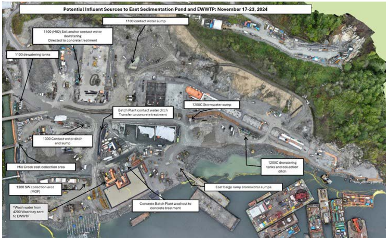
Figure 2: East Catchment contact water management facilities (November 17 – 23).
