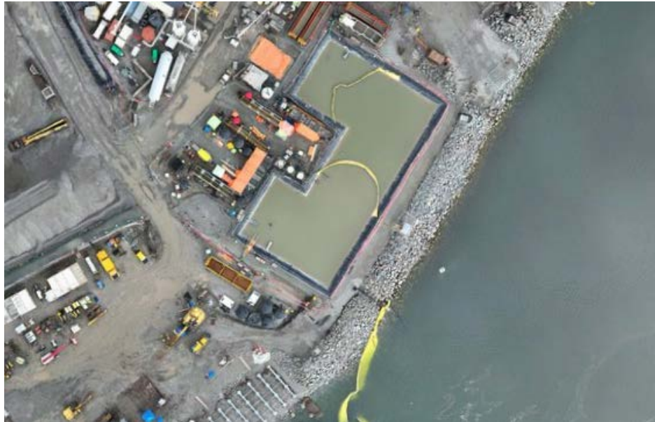
Figure 4: Aerial view of the East Sedimentation Pond showing the placement of two sediment curtains (October 25, 2024). The East WWTP is located on the left side of the pond.
