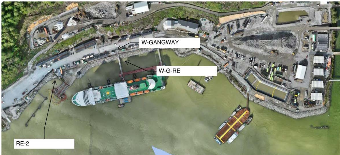
Figure 6: Location of pooled road surface stormwater sampled at West Gangway on October 19 (station W-GANGWAY) and locations of turbid site runoff observed in Howe Sound (stations W-GW-RE and RE-2) on October 19 and sampled October 19 and 20. The high turbidity plumes at W-GW-RE and RE-2 on October 19 were estimated to cover areas of approximately 1700 m 2 and 500 m 2 , respectively.
