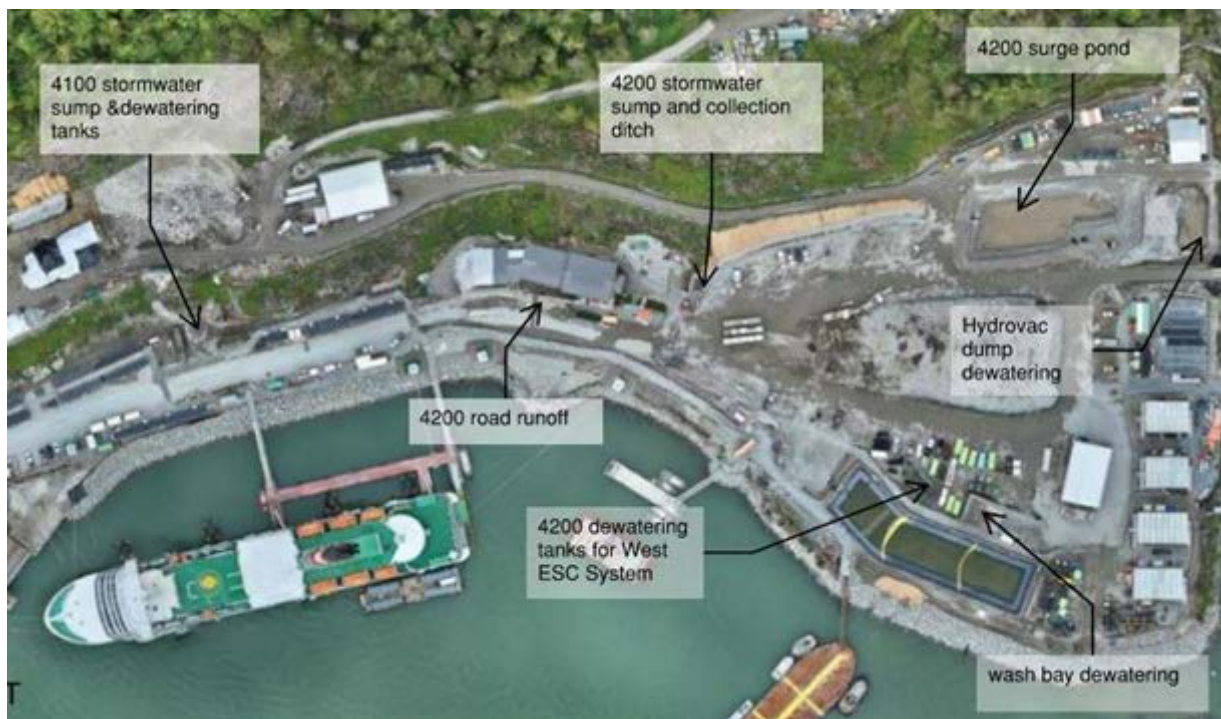
Figure 3: West Catchment contact water management facilities (October 20 – 26).
