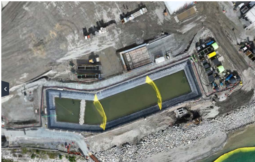
Figure 5: Aerial view of the West Sedimentation Pond showing the placement of two sediment curtains (October 2, 2024). The West WWTP is located on the right side of the pond.
