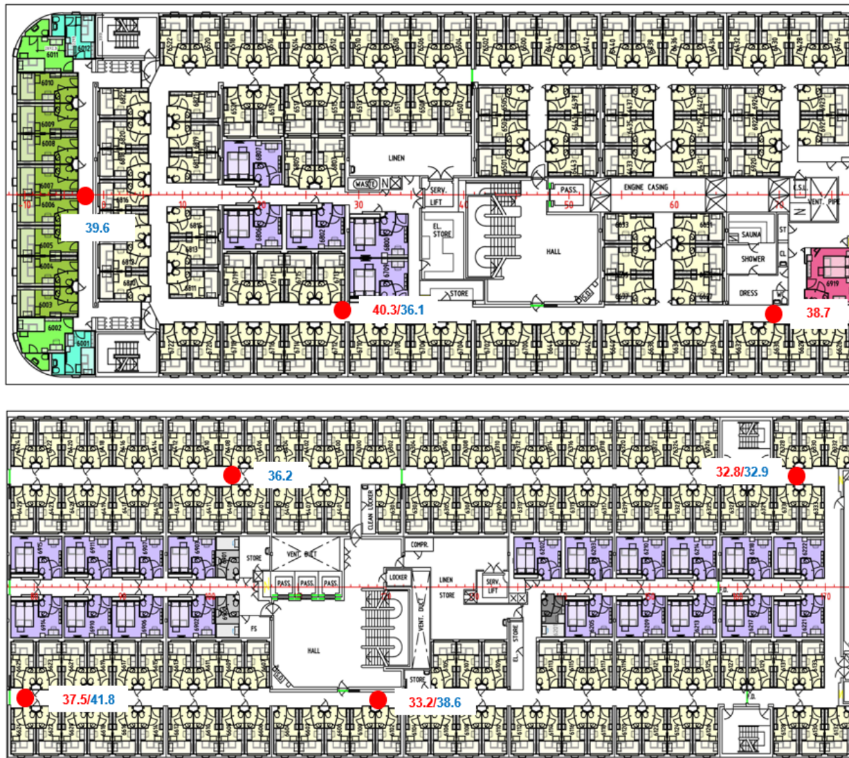
Figure 15: Spot Measurement Locations and Sound Levels – Deck 6
