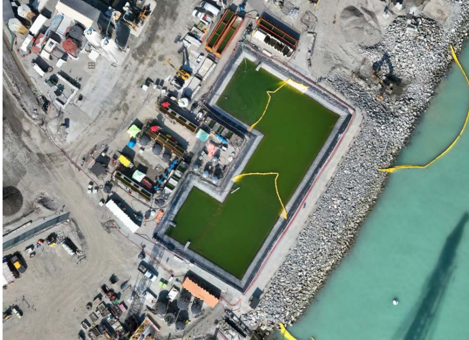
Figure 4: Aerial view of the East Sedimentation Pond showing the placement of two sediment curtains (September 6, 2024). The East WWTP is located on the left side of the pond.
