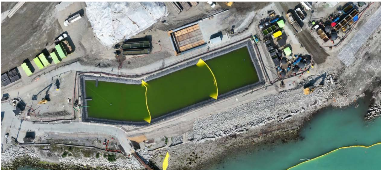
Figure 5: Aerial view of the West Sedimentation Pond showing the placement of two sediment curtains (September 6, 2024). The West WWTP is located on the right side of the pond.
