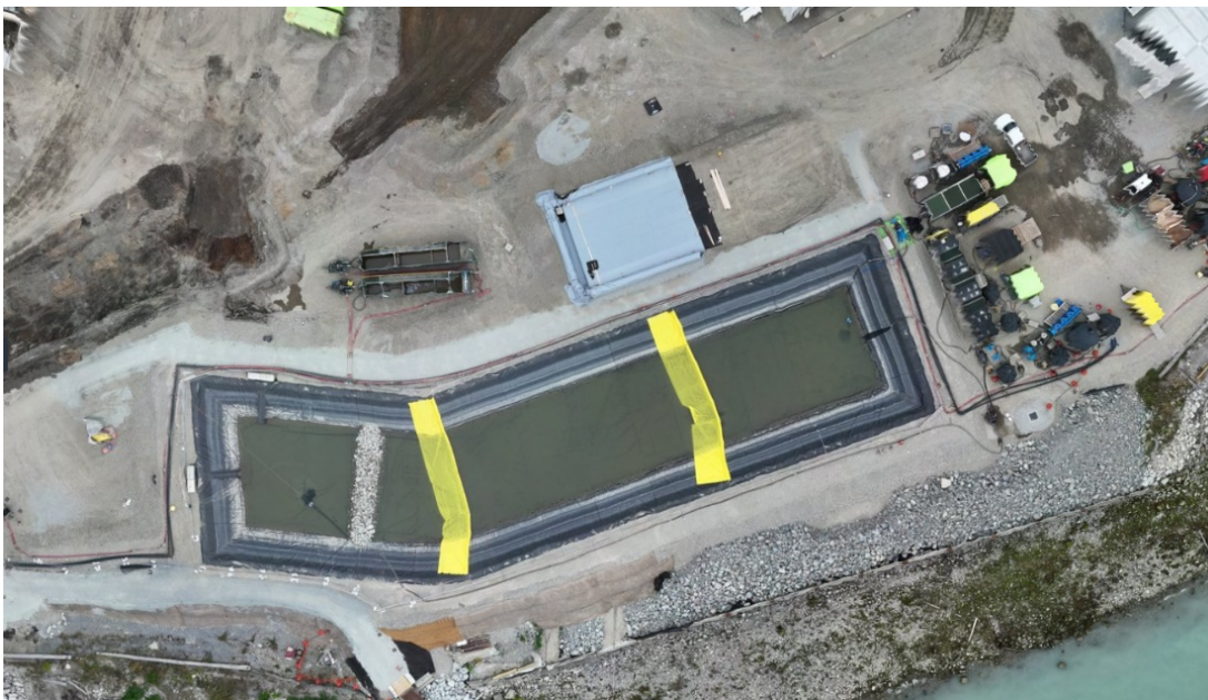
Figure 5: Aerial view of the West Sedimentation Pond showing the placement of two sediment curtains (August 16, 2024). The West WWTP is located on the right side of the pond.
