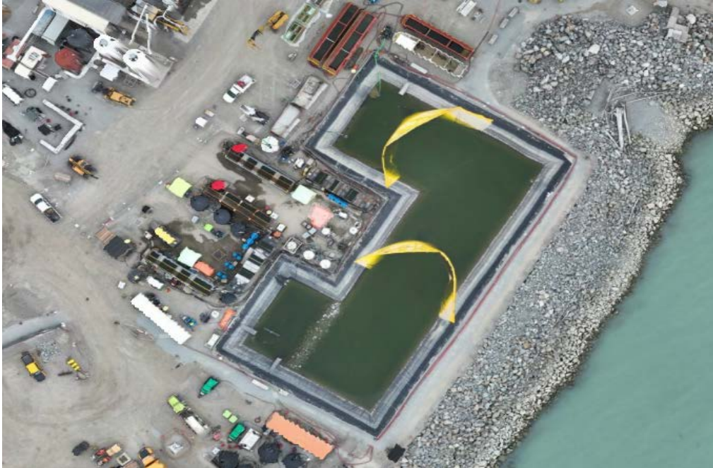
Figure 4: Aerial view of the East Sedimentation Pond showing the placement of two sediment curtains (August 16, 2024). The East WWTP is located on the left side of the pond.
