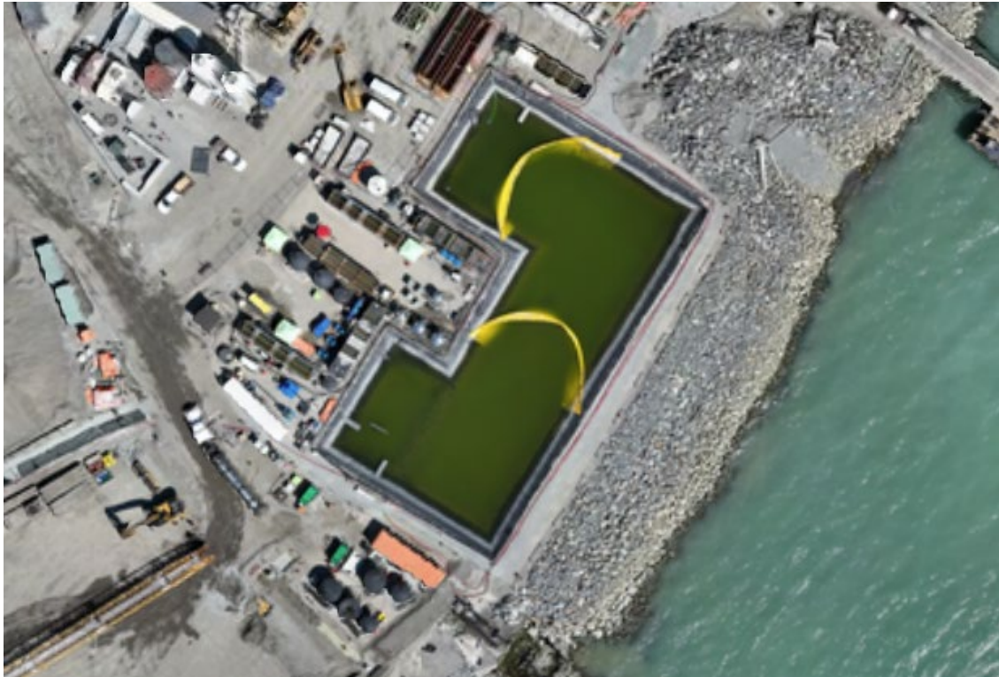
Figure 4: Aerial view of the East Sedimentation Pond showing the placement of two sediment curtains (July 19, 2024). The East WWTP is located on the left side of the pond.
