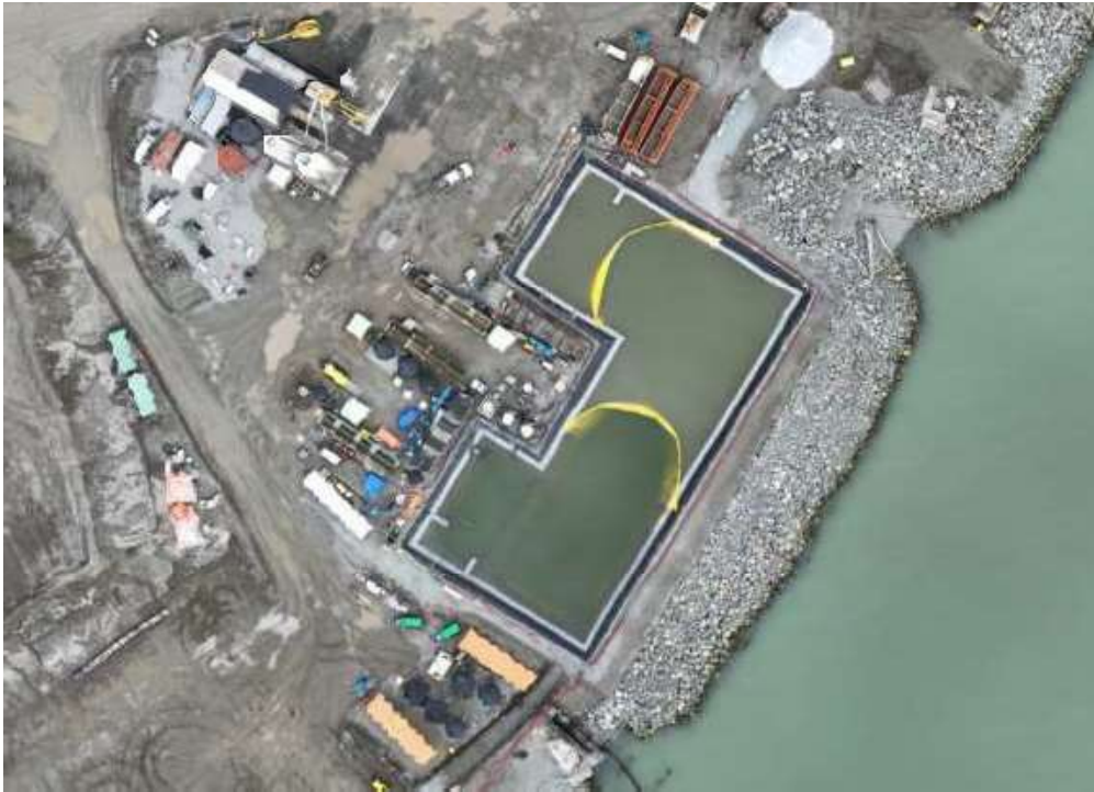
Figure 4: Aerial view of the East Sedimentation Pond showing the placement of two sediment curtains (June 28, 2024). The East WWTP is located on the left side of the pond.
