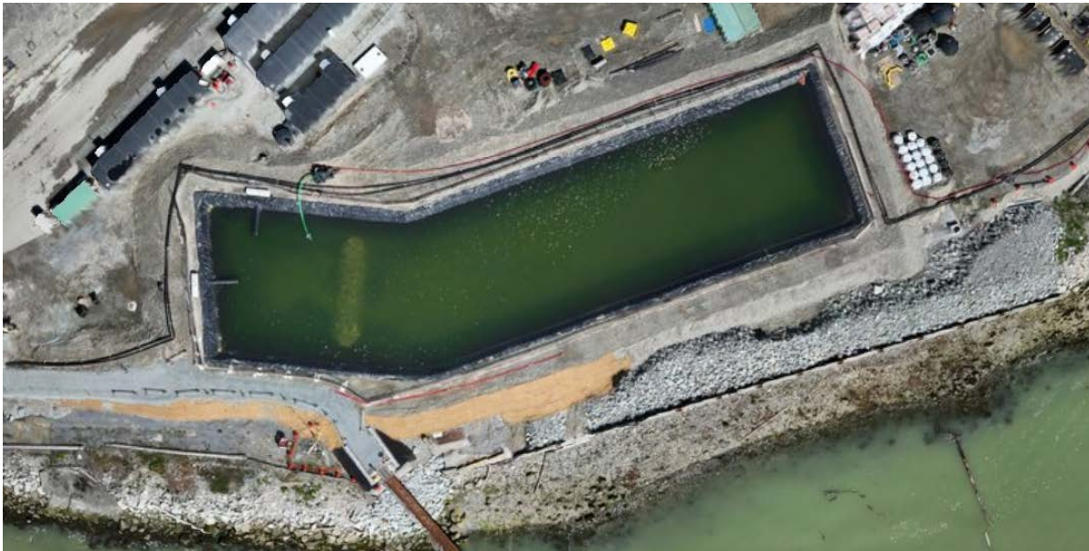
Figure 3: Aerial view showing the current stage of construction for the West Sedimentation Pond and West WWTP (located west of pond) on May 17, 2024. Water from the East Sedimentation Pond was transferred to the West Sedimentation Pond on May 13 – 15 to accommodate the clean-out of sediment at the bottom of the East Sedimentation Pond.
