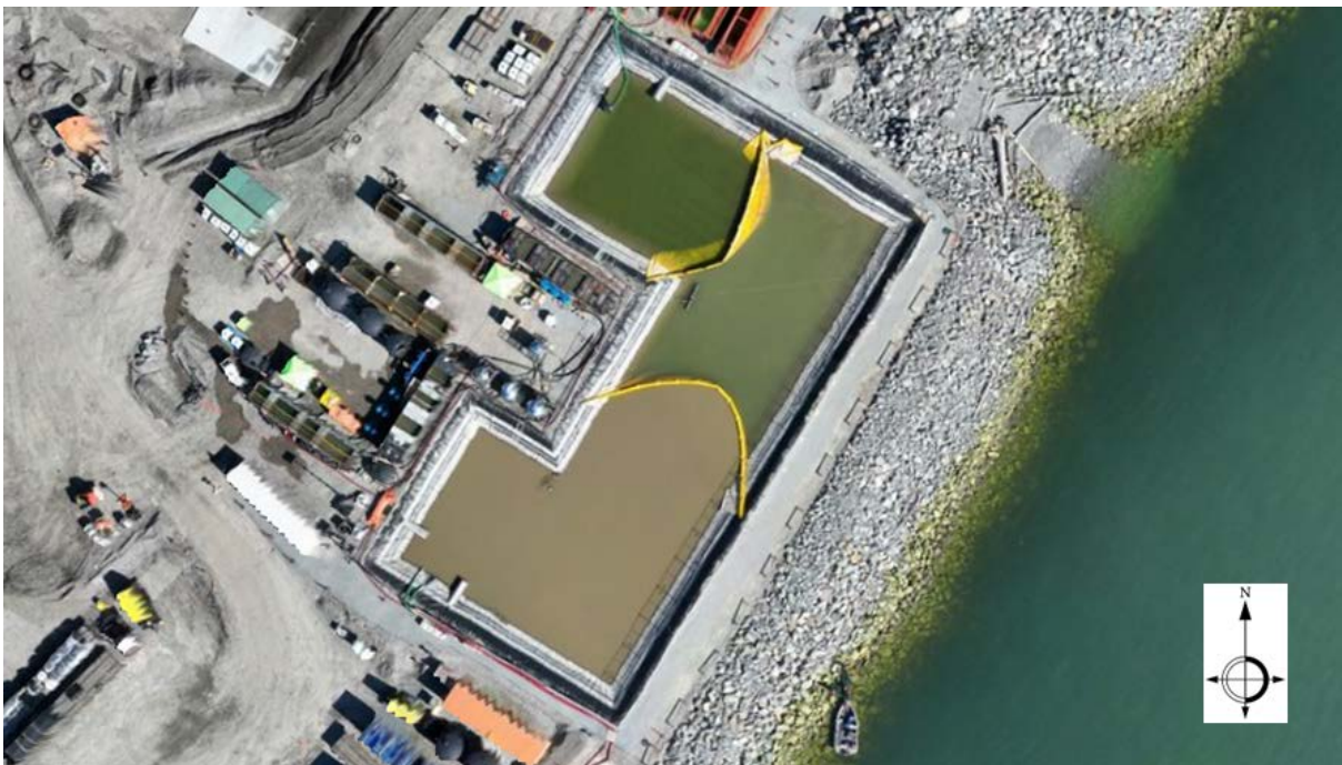
Figure 3: Areal view of the East WWTP and East Sedimentation Pond showing the placement of two sediment curtains. Water at the inlet (southwest) section of the pond is brown due to elevated TSS in the influent. The progression to clear water at the outlet (northern) end illustrates how TSS is held back by the curtains while allowing clarified water to pass through (April 19, 2024).
