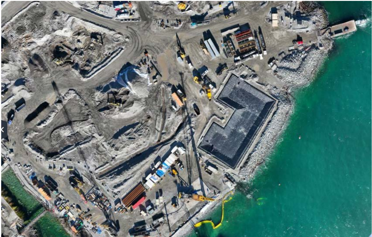
Figure 2: Areal view of the southern portion of the East Catchment showing the lateral extent of the East Sedimentation Pond (16-Feb-2024).
