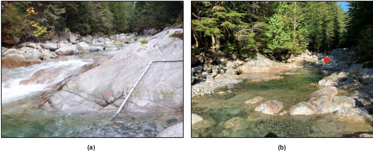
Photo 3 – (a) MILL-R2 Station looking upstream at the pressure transducer (October 2, 2019), and (b) looking upstream showing the Hydraulic Control (Aug 14, 2019). The gauge location is identified by the red dot.
