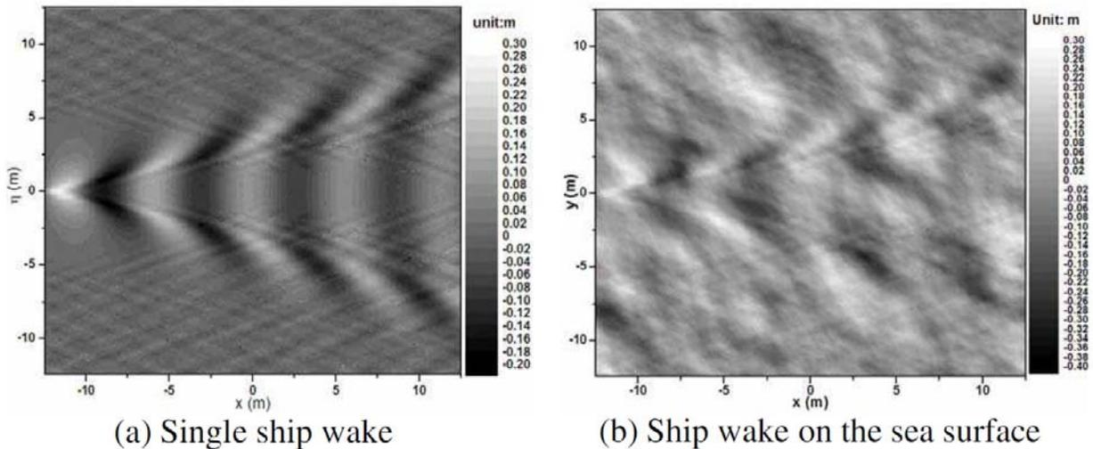
Figure 3 Example wake formation on calm water (a) compared with wake on sea surface (b).
