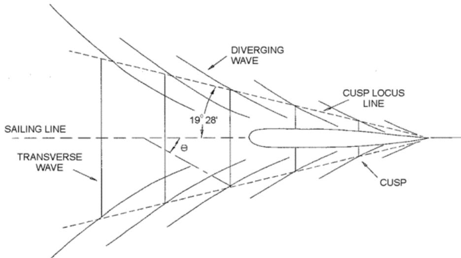
Figure 2 Vessel wake pattern.
