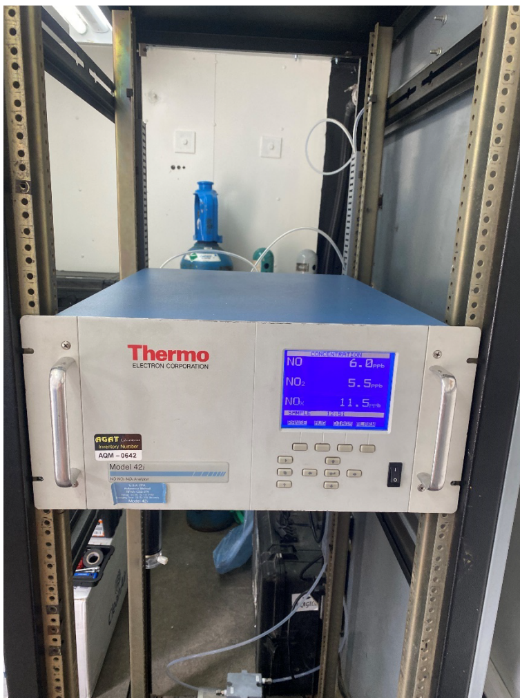
Photo 3.2 Thermo Scientific Model 42i (NO-NO 2 -Nox) Gas Analyzer at the Woodfibre LNG AQMS
